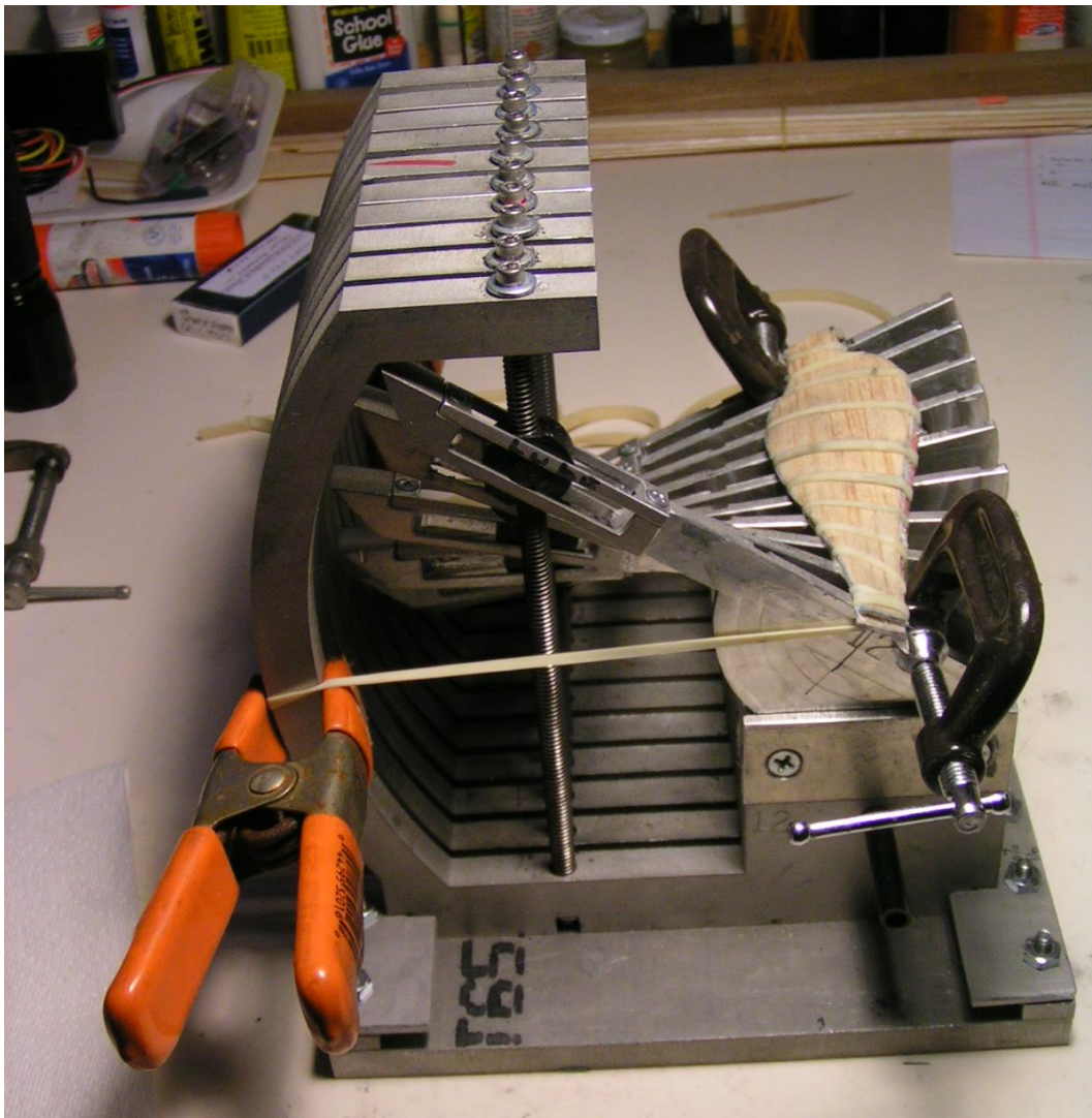
Figure 8 – Machined Prop Molding Jig in Use
