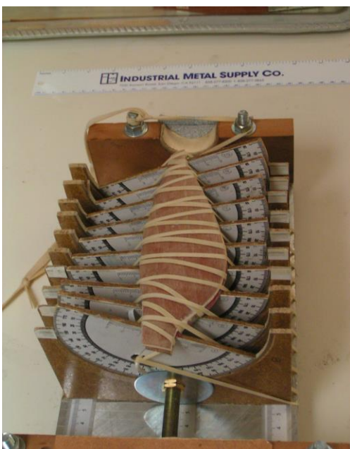
Figure 1 - Larrabee 12" diameter prop blade on jig
