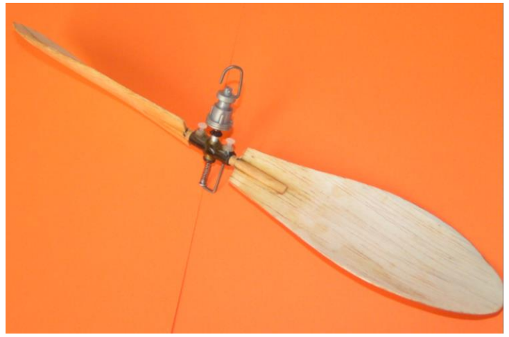
Figure 7 – 12” Fiber-glassed Balsa Prop Assembly
