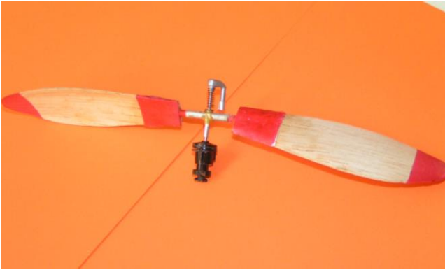
Figure 6 – 10” Molded Balsa Prop Assembly
